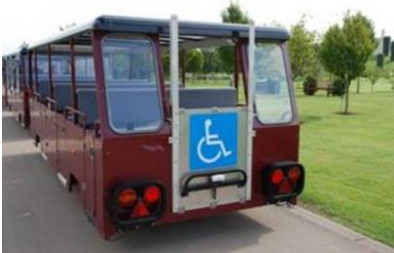
Land train access ramp in stowed position
