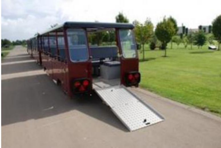
Land train access ramp
